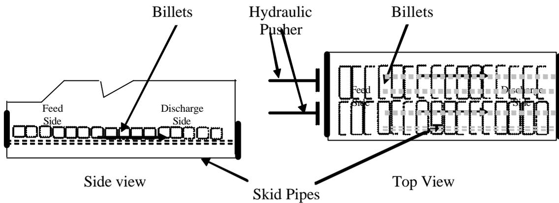
**Figure 1- Billet Heating Furnace - Schematic**
