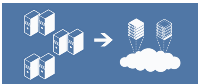
Consolidating virtualized applications onto shared hardware increases the utilization of server resources.
