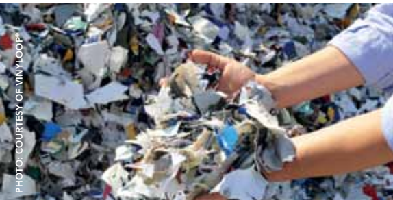
PVC coated fabrics waste from Serge Ferrari ready to be recycled at the VinyLoop ® plant in Ferrara, Italy
